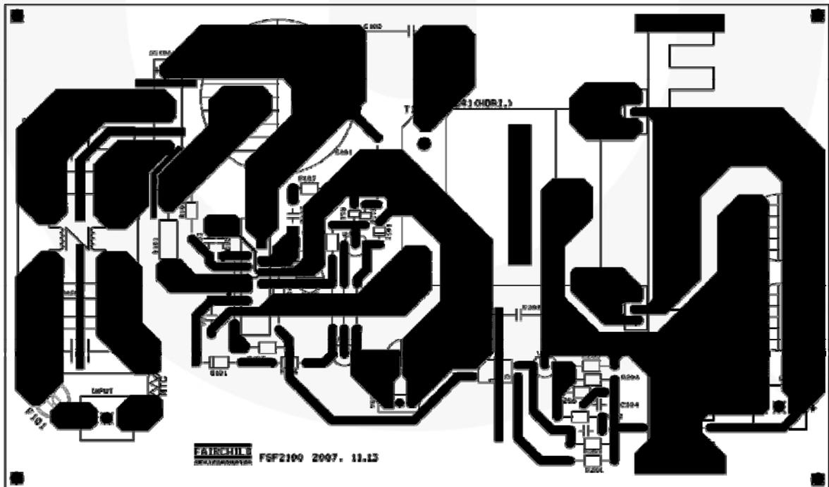
Figure 5. Bottom PCB Image of the Evaluation Board
