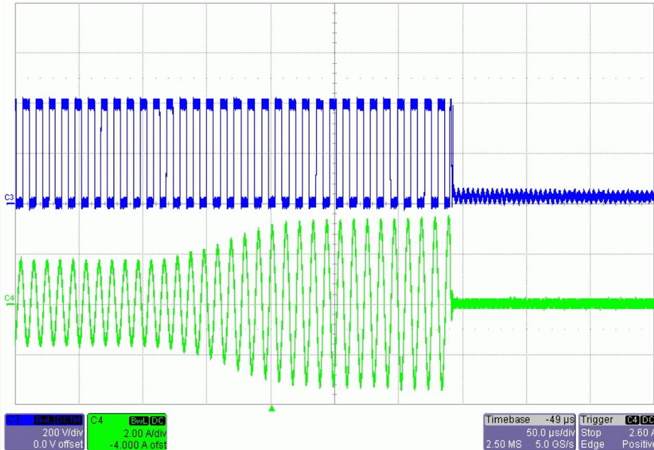
**Figure 21. Protection Waveform at Overload Condition [ $V_{IN}=390V_{DC}$ , ( $I_o=8A \rightarrow 16A$ )]**
