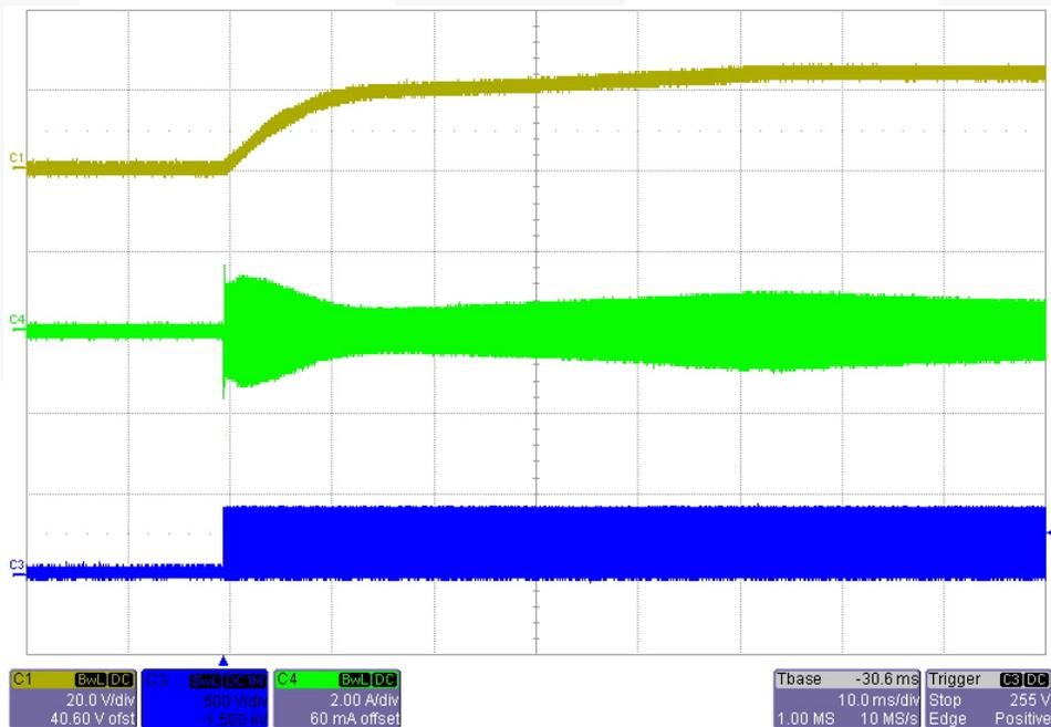
**Figure 15. Start-up Waveforms at Nominal Input Voltage [ $V_{IN}=390V_{DC}$ ,  $P_O=0W$  (24V/0A)]**
