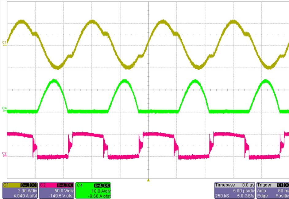
**Figure 11. Operation Waveforms at Minimum Input Voltage [ $V_{IN}=340V_{DC}$ ,  $P_O=192W$  (24V/8A)]**
