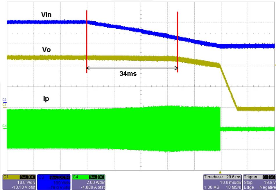
**Figure 20. Output Voltage Waveform after Turning Off Input Voltage [ $V_{IN}=390V_{DC}$ ,  $P_O=192W$  (24V/8A)]**
