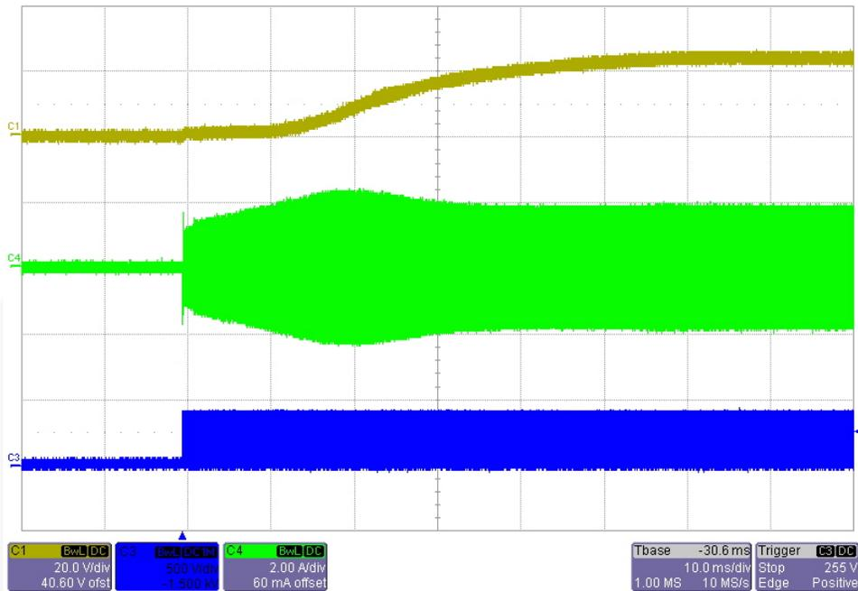
**Figure 14. Start-up Waveforms at Nominal Input Voltage [ $V_{IN}=390V_{DC}$ ,  $P_O=192W$  (24V/8A)]**
