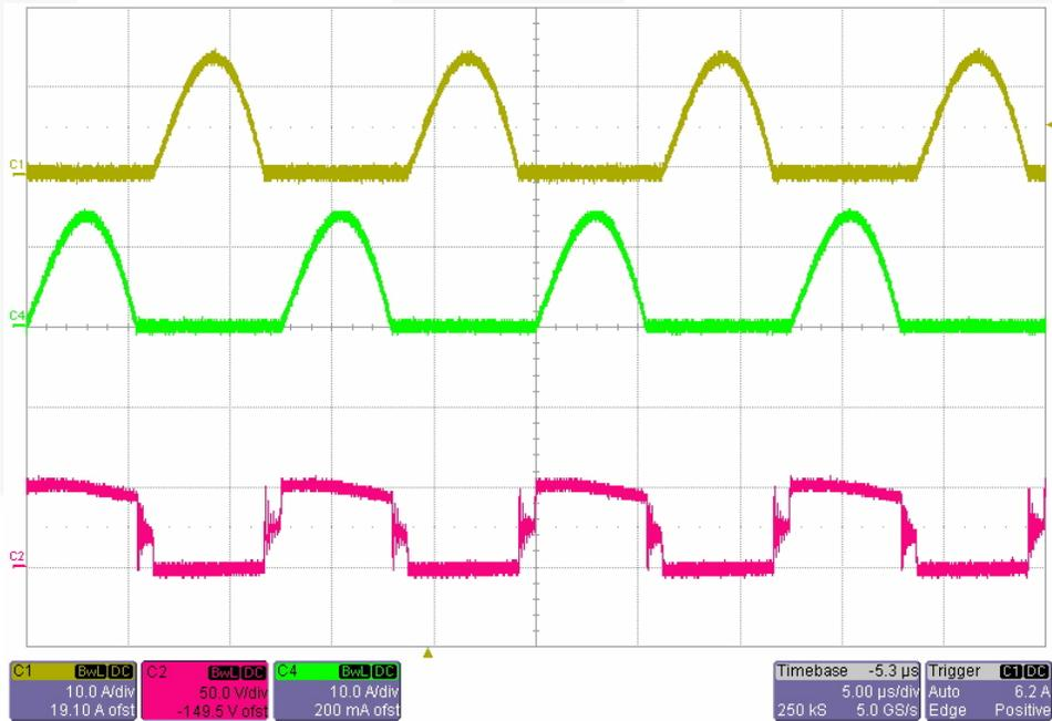
Figure 13. Operation Waveforms at Minimum Input Voltage [ $V_{IN}=340V_{DC}$ ,  $P_O=192W$  (24V/8A)]
