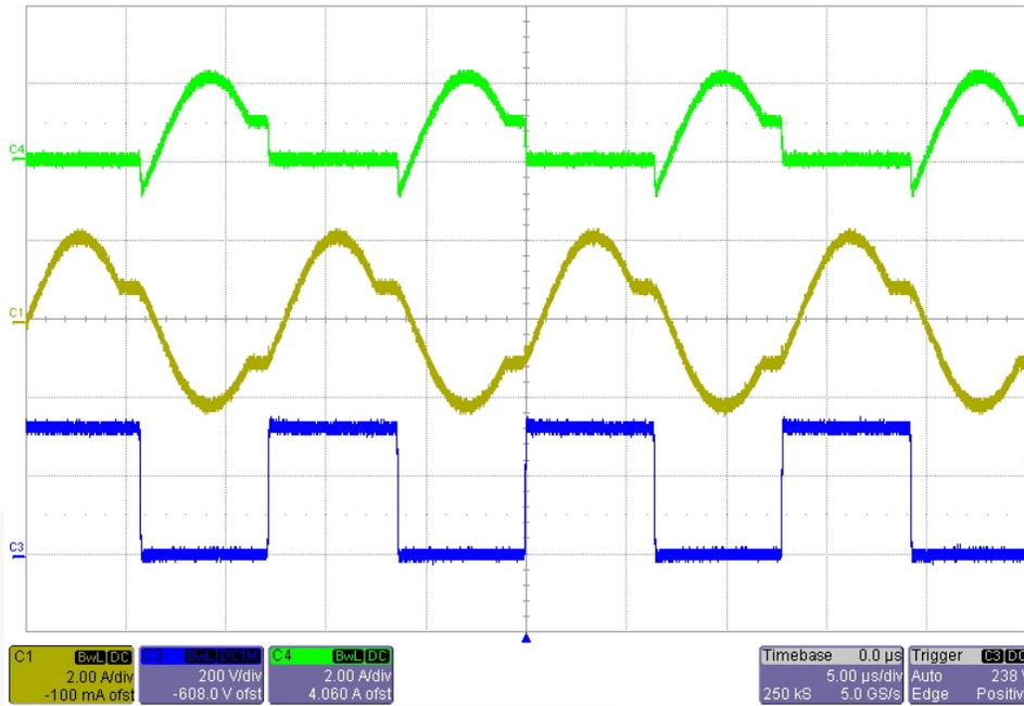
**Figure 8. Operation Waveforms at Minimum Input Voltage [ $V_{IN}=340V_{DC}$ ,  $P_O=192W$  (24V/8A)]**
