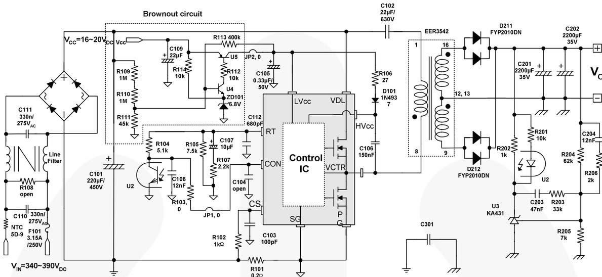
Figure 1. FSFR2100 Evaluation Board (LCC Resonant Converter)
