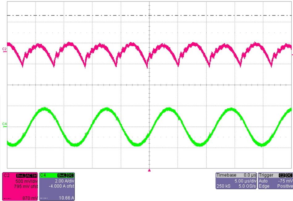
**Figure 18. Output Voltage Ripple at Nominal Input Voltage [ $V_{IN}=390V_{DC}$ ,  $P_O=192W$  (24V/8A)]**
