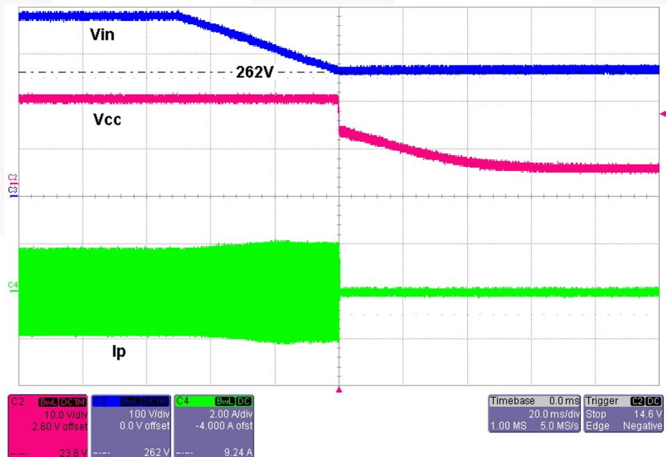
**Figure 17. Power-Off Waveforms at Nominal Input Voltage [ $V_{IN}=390V_{DC}$ ,  $P_O=192W$  (24V/8A)]**
