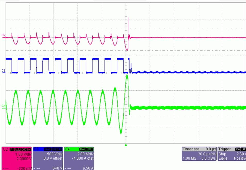
**Figure 22. Protection Waveform at Output Short Condition [ $V_{IN}=390V_{DC}$ , ( $I_o=8A \rightarrow$  Short)]**
