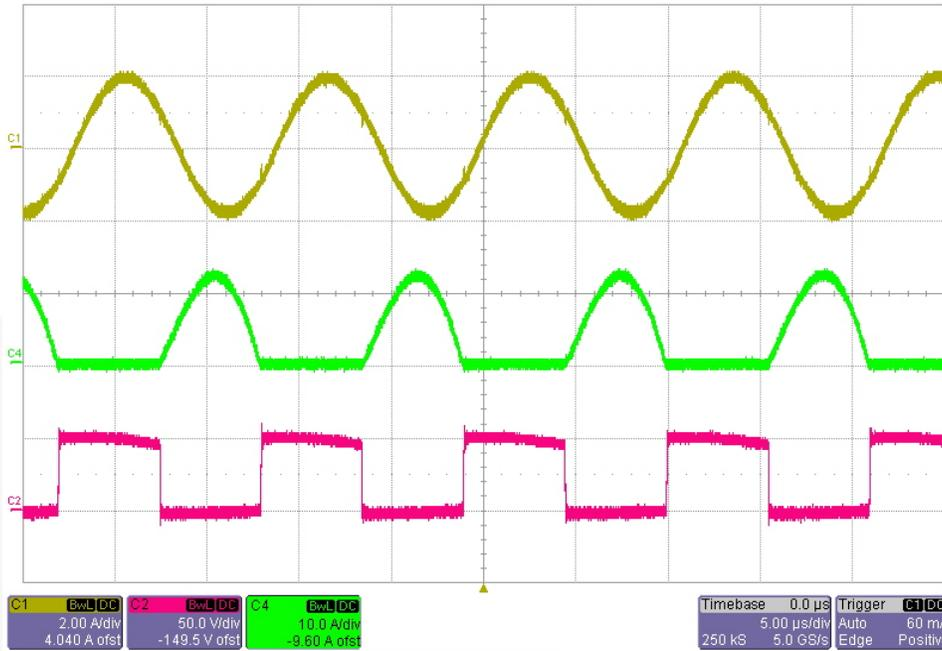
**Figure 10. Operation Waveforms at Nominal Input Voltage [ $V_{IN}=390V_{DC}$ ,  $P_O=192W$  (24V/8A)]**
