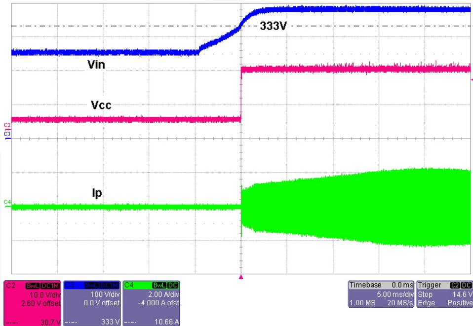
**Figure 16. Power-on Waveforms at Nominal Input Voltage [ $V_{IN}=390V_{DC}$ ,  $P_O=192W$  (24V/8A)]**
