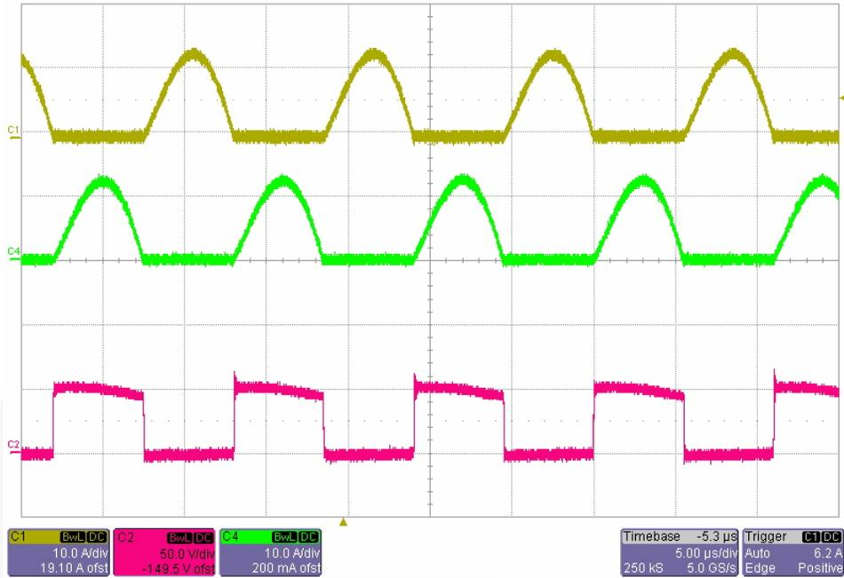
Figure 12. Operation Waveforms at Nominal Input Voltage [ $V_{IN}=390V_{DC}$ ,  $P_O=192W$  (24V/8A)]
