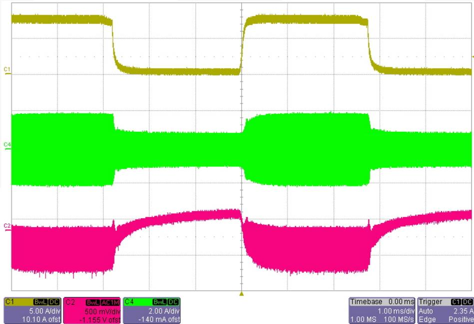
**Figure 19. Output Voltage Ripple with Pulse Load Current at Nominal Input Voltage**
