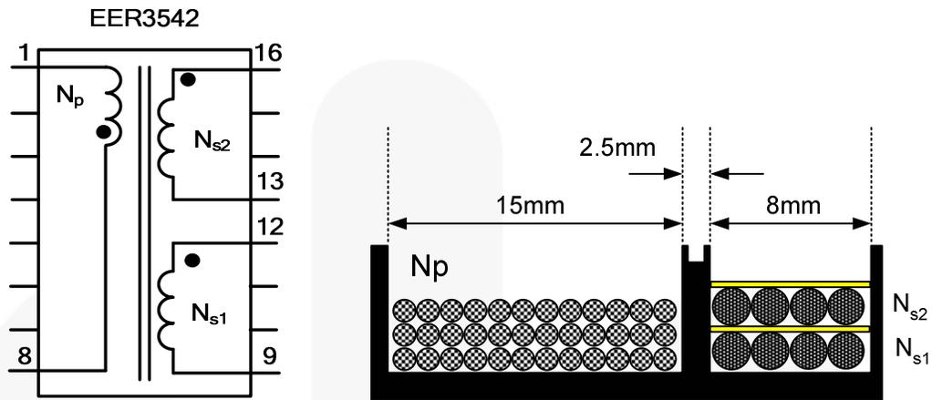
Figure 3. Transformer Specifications
