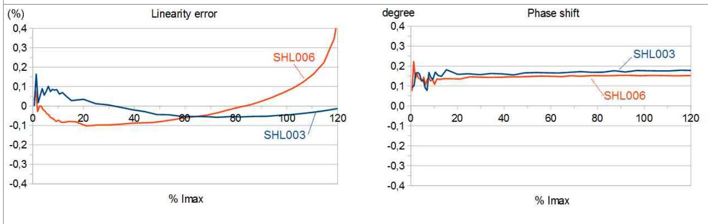
The showed errors and typical graphs are referred to 50/60Hz AC current measuring, Rb=10kΩ.
